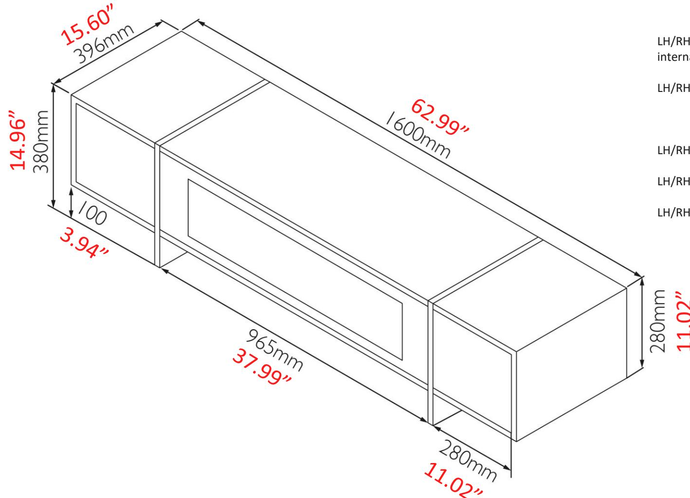
LH/RH compartment dims (WIDTH) | 258mm (10.16") including door thickness / 280 (11.02") internal compartment
